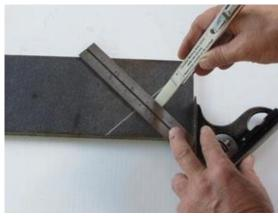
Where the ends of the lines meet the edge of the bar scribe a perpendicular line. A square has created its center marked where the diagonal lines cross.
