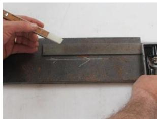
The steel rule can be slid through the head to set the face at an exact point. Layout lines short distances from edges can be quickly and precisely made this way.
